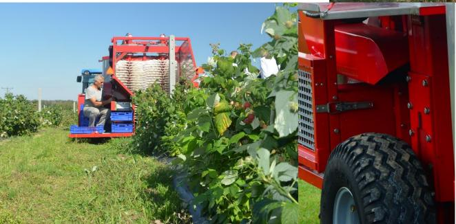
Harvester lifting on wheel columns ensures low harvester position during fruit harvesting, allows to work on slopes and overcome field obstacles.
