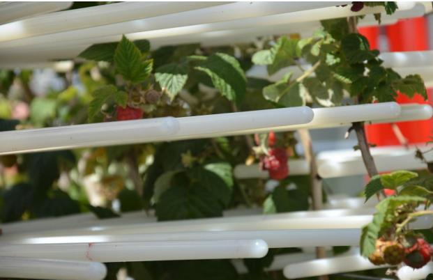
Vertical shakers and shaking rods configuration guarantees efficient fruit shaking even with gentle vibrations. Fast and easy regulation of shaking unit allows for wide range of working parameters change and adaptation to picking requirements. Only ripe fruit are shaking off. Unripe fruit are leaving and undamaged for the next pick.
